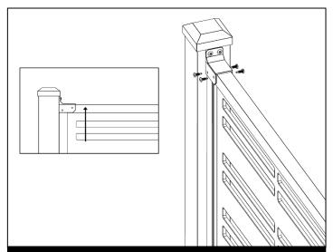
Step 8 - Attach Upper Horizontal Frame Channel
